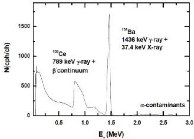
Figure 5. Background spectrum of the LaBr<sub>3</sub> detector used in our measurements
