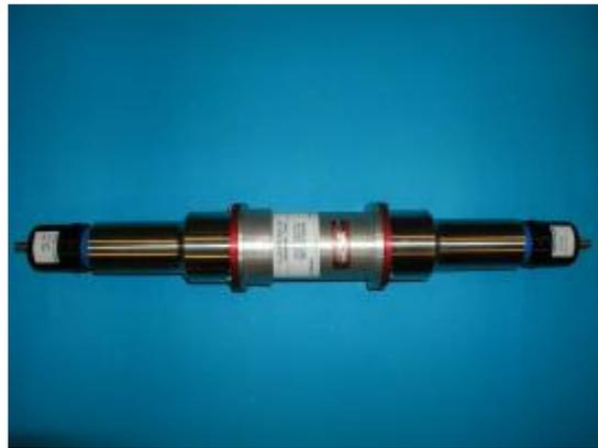
Figure 2. A 15cm long, 7.5 cm diameter test cell, sandwiched between two PMTs.
