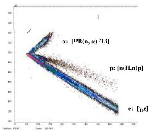
Figure 3. PSD with the EJ309 scintillation liquid. For the interpretation of the loci see text.
