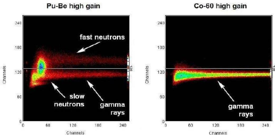
Fig.2. Differences in pulse shape between neutrons and gamma-radiation for a cell filled with EJ309-5% <sup>nat</sup>B. The figure the zero-crossing is plotted as function of energy, both in arbitrary units. (obtained from IPN. Warsaw)
