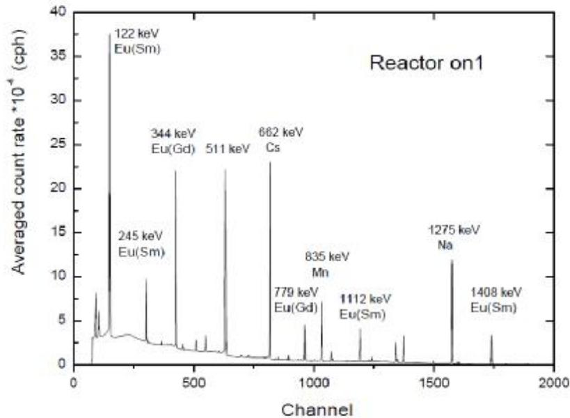
Fig. 4: Hourly gamma-ray spectrum averaged over reactor-on1 period.
