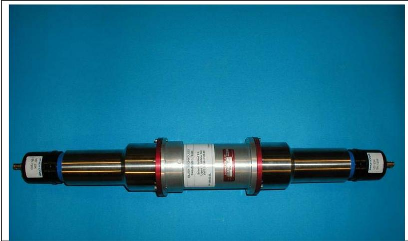
Figure 3. A test cell filled with liquid scintillator equipped with two PMTs
