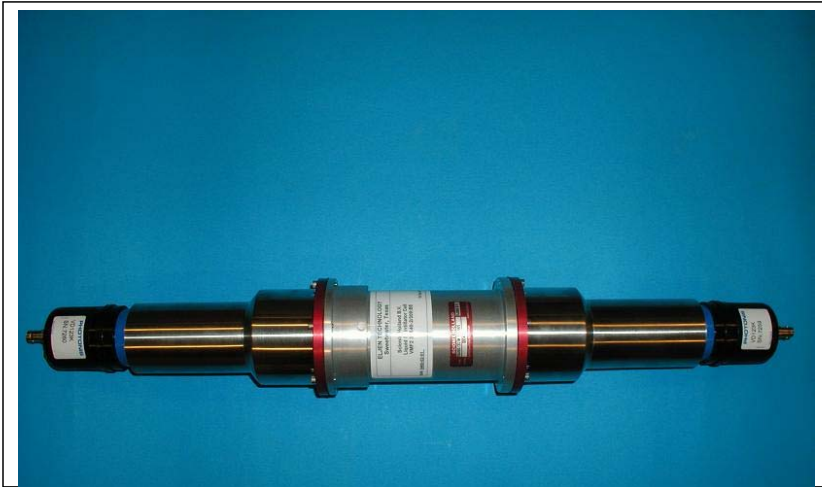
Figure 3. A test cell filled with liquid scintillator equipped with two PMTs
