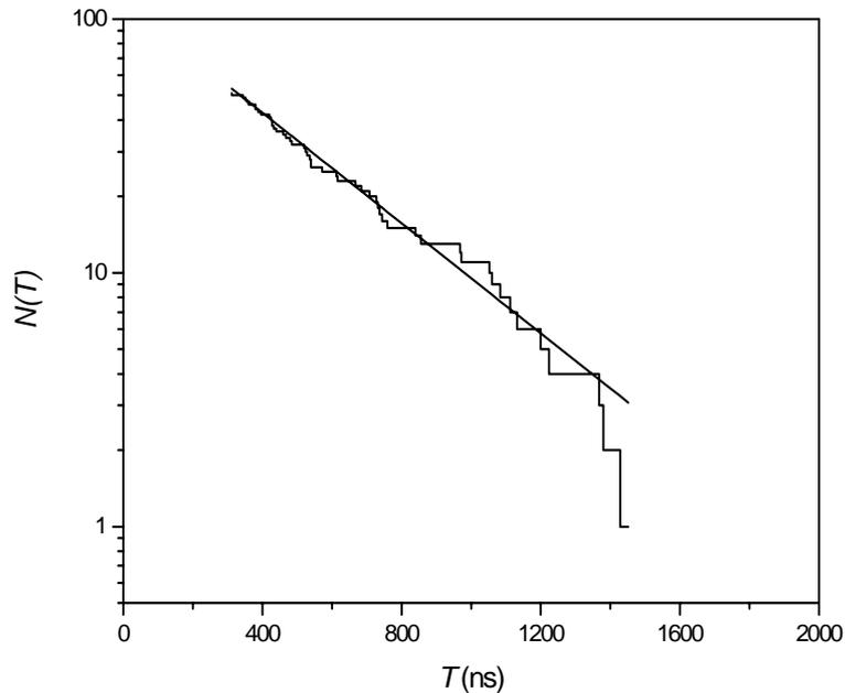
Figure 1: Plot of  $N(T)$ , the number of events for which the time delay between first and second pulses is  $\geq T$ , versus  $T$ . The histogram shows experimental data obtained using neutrons from a  $^{252}\text{Cf}$  spontaneous fission source. The line shows the fitted function  $N(T) = 116 \exp(-T/T_0)$  for  $T_0 = 400$  ns.
