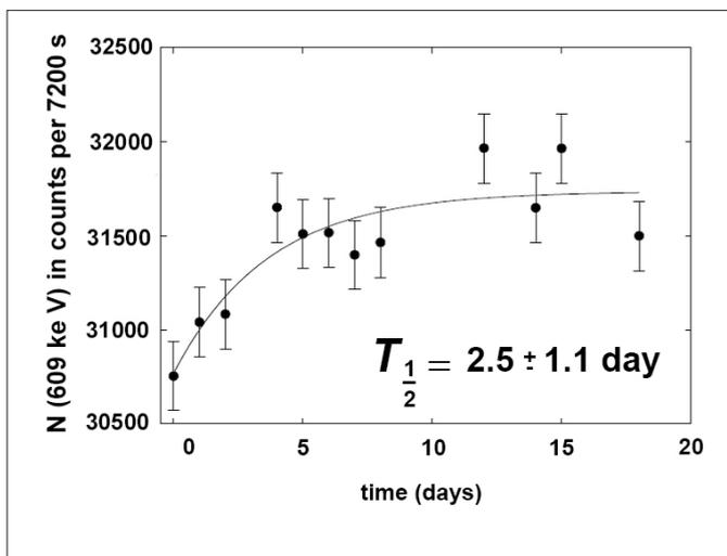
Figure 5 Count rate in the  $E_{\gamma}=609 \text{ keV}$  line of  $^{238}\text{U}$ -decay series as function of time since sealing sample #13a.
